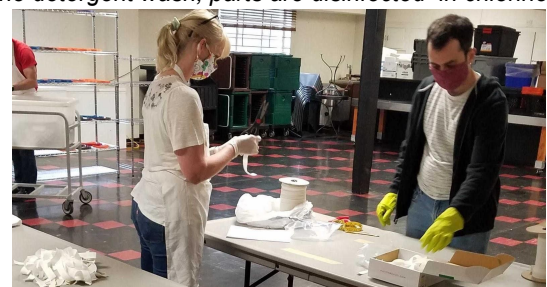
The face shields have multiple parts: headbands, chins, elastic straps (being fabricated here), clear plastic visors, and printed instructions.
